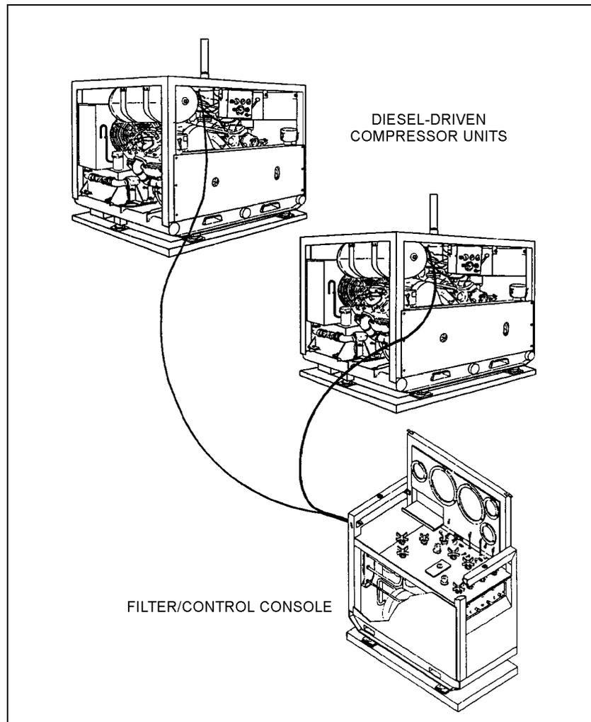
Figure 8-8. Flyaway Air Diving System (FADS) I.
