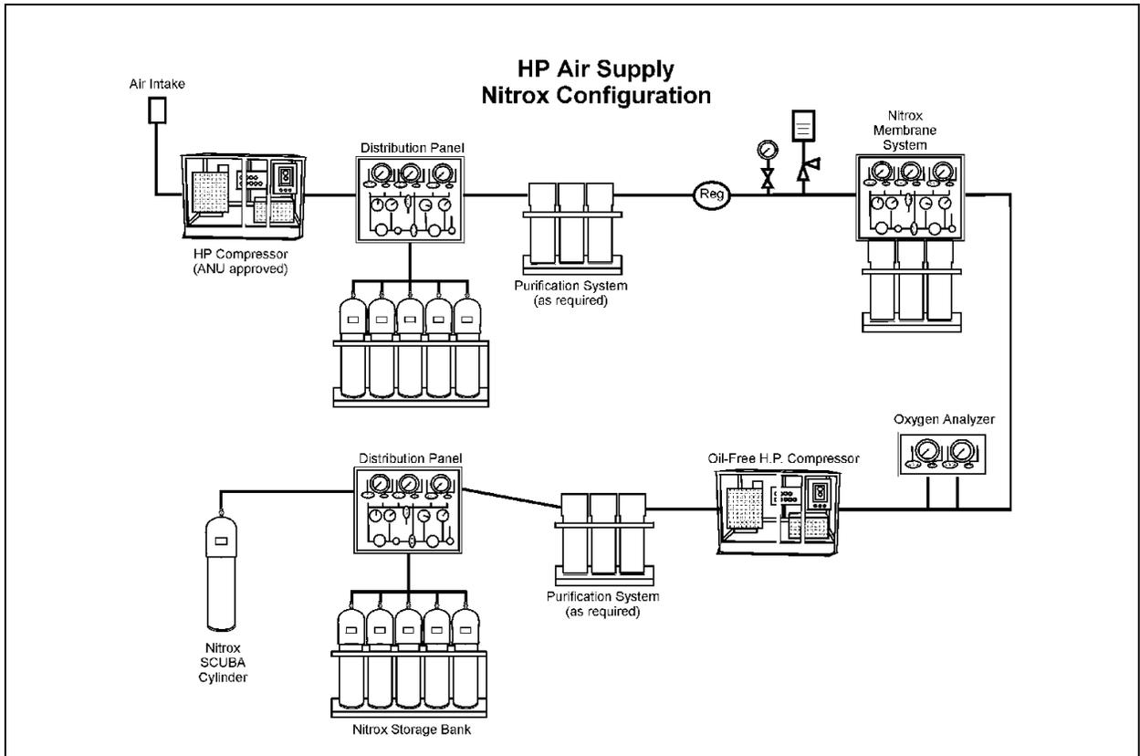
**Figure 10-5.** HP Air Supply NITROX Membrane Configuration.
