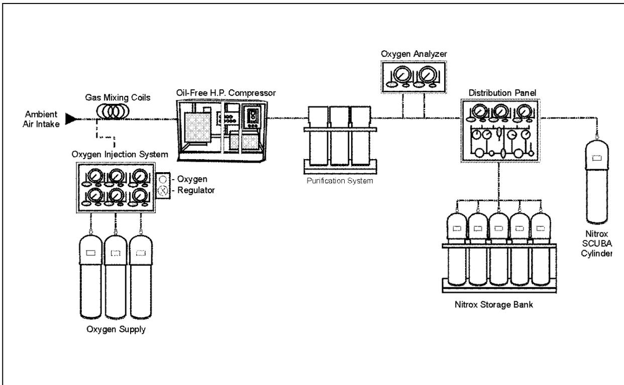
Figure 10-3. Nitrox O<sub>2</sub> Injection System.
